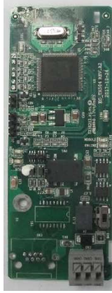
CANopen/CAN master/slave control communication card EC-TX505/511
